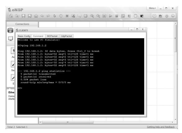
The generation of traffic will be confirmed by the resulting output in which case the number of packets transmitted are shown to also be received.
