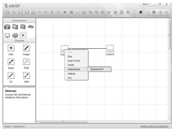
The selection of an interface will result in the activation of the Wireshark packet capture tool for the selected interface. If additional interfaces are to be monitored, separate instances of the same packet capture tool will be activated.
