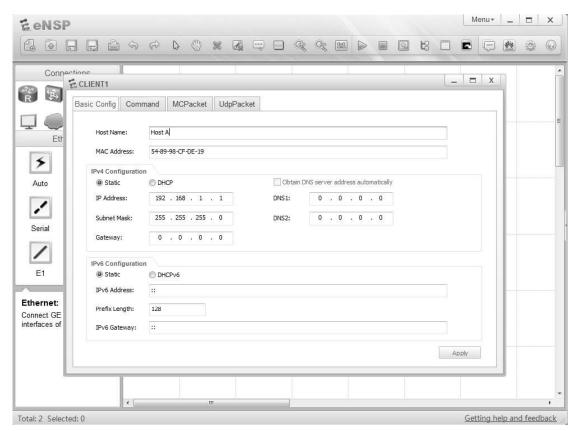
The same process is required for CLIENT2. It is recommended that initially the IP address 192.168.1.2 be configured, with a subnet mask of 255.255.255.0.
