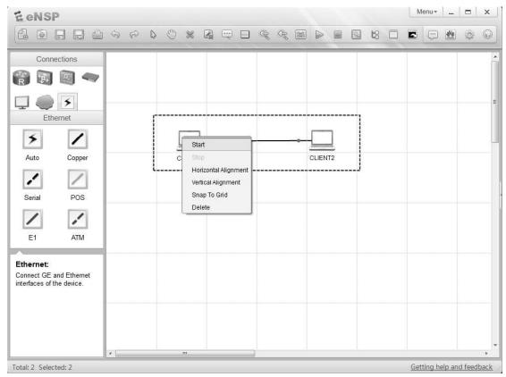
Once the devices are online and active, it is common to notice a change in the status of the connectors through a switch in the colour of the red dot on the medium to green, highlighting that the status of the connectors is now up.
