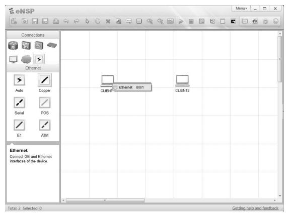
Once this has been achieved, click on the peering device to apply the opposite end of the medium to the end system. Again select the interface Ethernet 0/0/1 to establish the medium between the two devices and complete the construction of a peer-to-peer topology.
